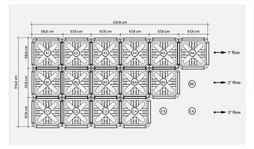
To ensure a correct installation and perfectly created under-floor cavity please refer to the product's usage requirements.
