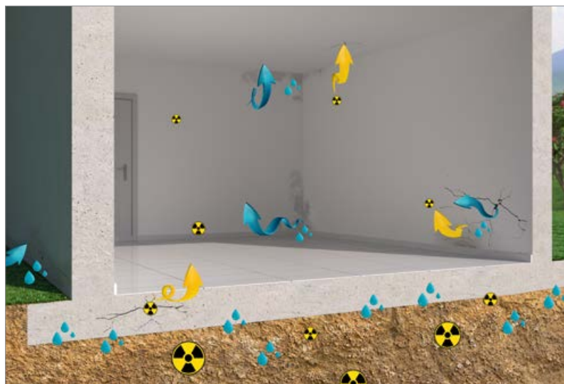
Danger of Radon gas and rising humidity in a home built on a traditional foundation.
