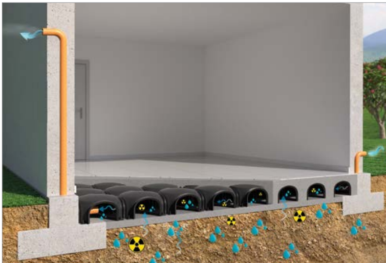
Home built with a ventilated IGLU® foundation.
