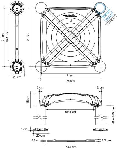
Atlantis 71x71 System includes, for each square meter, 2 formworks, 2 pipes, 2 feet (and 4 optional spacers).
