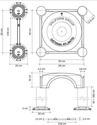
Atlantis 50x50 System includes, for each square meter, 4 formworks, 4 pipes, 4 feet (and 8 optional spacers).
