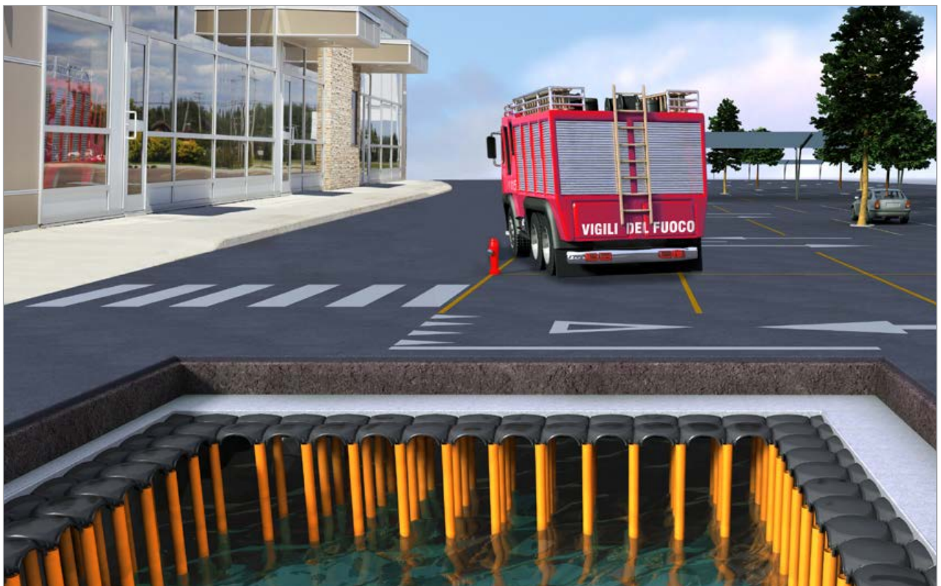
Collection tank used as a fire extinguishing system
