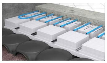
4 Lay the finishing slab foundation reinforcements and the reinforcements inside the ribbing. Then, cast the concrete in the ribbed slab foundation which should be well beaten down (especially along the sides and in the corners), compacted across its full thickness, supported and trowelled (by hand or using a trowelling machine) to a professional standard. After waiting for the concrete to mature, lay the flooring as per the design.
