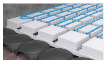
3 Lay any pipe coils for the underfloor heating and cooling system, fastening them to the Iso Iglu" panels using the relevant clips for radiant underfloor heating systems. Any other system pipes can be inserted inside the orthogonal channels.
