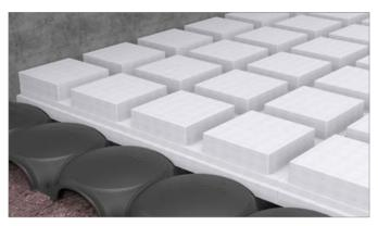
2 Lay the Iso Iglu" panels in EPS, taking care to position them so that the intrados shaping of the Iso Iglu" matches up perfectly with the extrados of the Iglù Plus domes.
