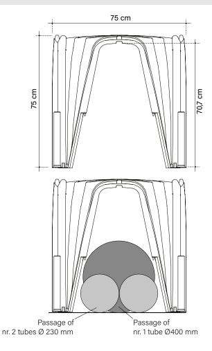
The images are only for examples. Recyclable material is allowed a size tolerance of  $\pm$  1,5%.
