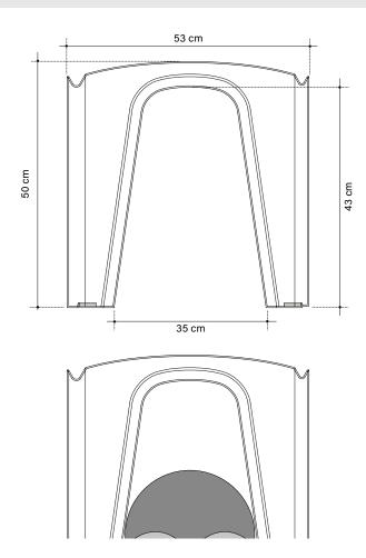
The images are only for examples. Recyclable material is allowed a size tolerance of  $\pm$  1,5%.
