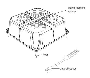
The images are only for examples: reinforcement spacers can have different shapes and positions. Recyclable material is allowed a size tolerance of  $\pm$  1,5%.
