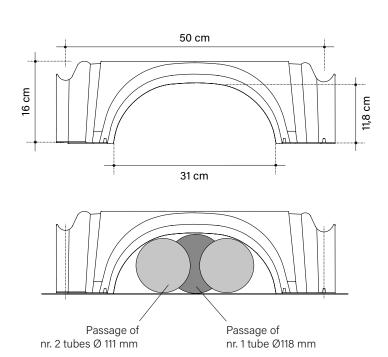
The images are only for examples. Recyclable material is allowed a size tolerance of  $\pm$  1,5%.
