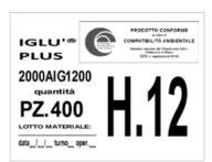
A lebel with the following informations: product's name and code, quantity, Certificate of the Environmental Compatibility, date of production, shift of production, n° of the worker, production line batch.
