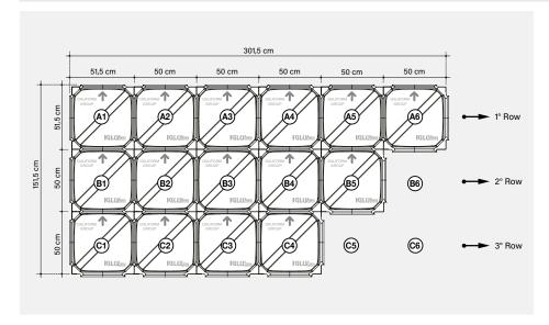
To ensure a correct installation and perfectly created under-floor cavity please refer to the product's usage requirements.
