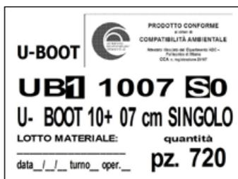
A label with the following informations: product's name and code, quantity, Certificate of the Environmental Compatibility, date of production, shift of production, n° of the worker, production line batch.
