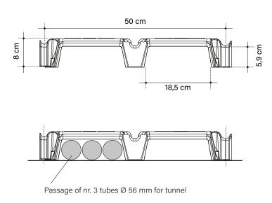
The images are only for examples. Recyclable material is allowed a size tolerance of  $\pm$  1,5%.
