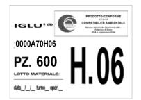
A lebel with the following informations: product's name and code, quantity, Certificate of the Environmental Compatibility, date of production, shift of production, n° of the worker, production line batch.
