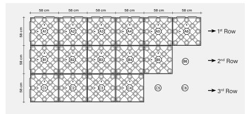
The IGLU'® Green Roof panels are connected through special clips, which give stability and ability to adapt even on curved surfaces.
