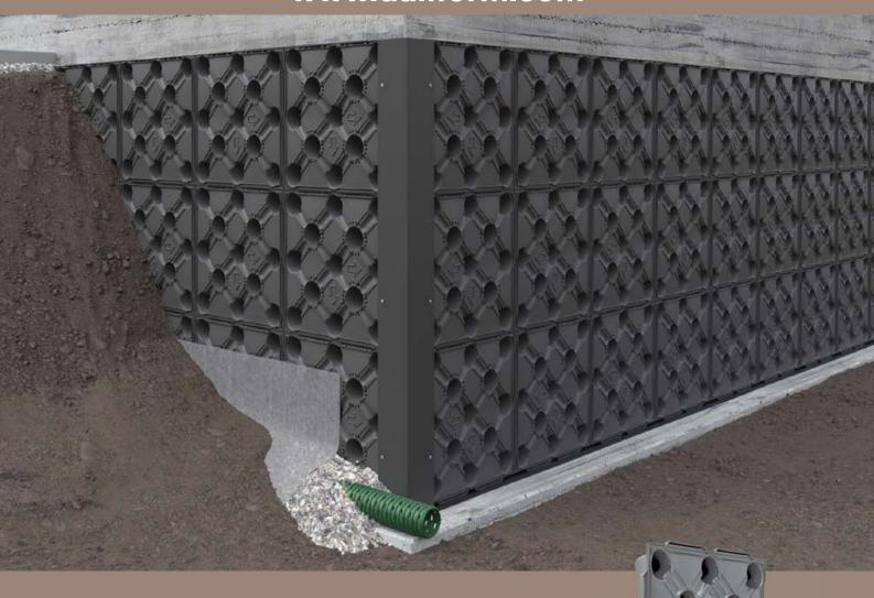
Protection of the waterproof in retaining walls
