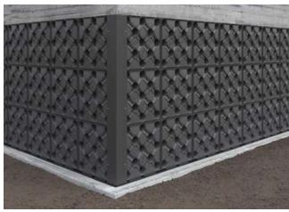
Place the angle closing as to avoid infiltrations by attaching it to the Iglu'® Barrier panel with screws or chemical plugs no longer than 3cm (this prevents drilling the waterproofing).
