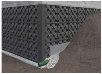
Cover the draining pipe with scree and then with geotextile. After that, proceed with the backfill.
