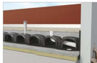
Systems for sloped or flat ventilated roofs IGLU® VENTILATED ROOF
