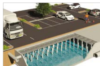
Systems for underground collection tanks IGLU®, SISTEMA ATLANTIS TANK
